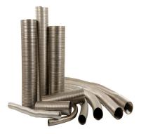
**FUMIFLEX** — Flexible hose in shape like can volute made by high — allayed stainless steel strip in quality acc. to USA standard AISI 304, assembled by double strip wounded. Lead of helix double strip wound enable its high-leak profess and good flexibility, small weight and economical.
